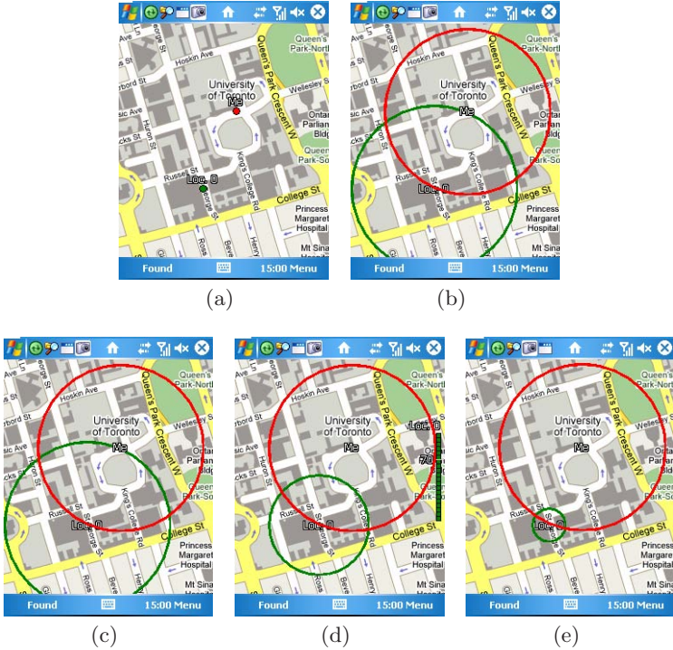
Fig. 3. The experimental four conditions: predicted location (a); 95% confidence (b); customizable confidence by default (c) and after the confidence value has been manipulated (d); and optimal error (e)
