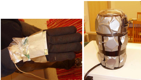
Fig. 1. (l) The glove with an RFID reader attached. (r) The coffee grinder with several RFID tags attached.
