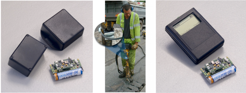
Fig. 3. Sensor-based vibration monitor system with wireless drill & dosimeter (reproduced from [7])
