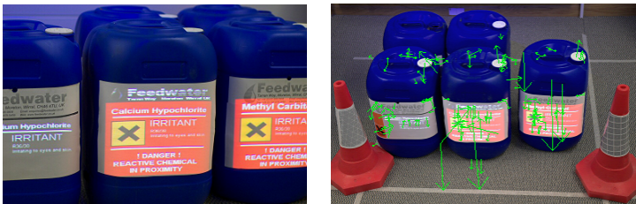
Fig. 6. Left: Warning message projection on two chemical containers, Right: Scale and rotation invariant local features detected on chemical containers
