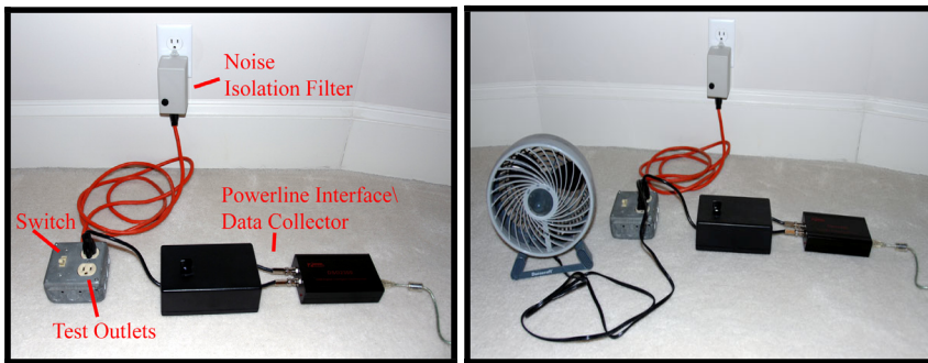
Fig. 7. The setup we constructed for isolating and testing the noise response for various electrical devices on an individual basis
